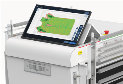
1. RED-GREEN COLORING, HIGHLIGHTING THE CONDITION OF PPE
